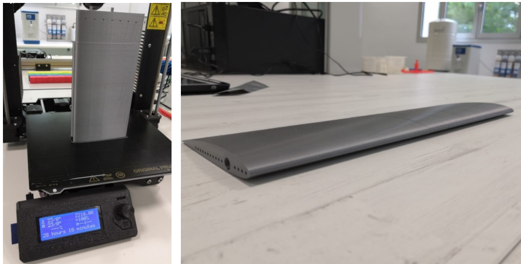
Figure 3: NACA 2412 airfoil 3D printing (28h 18') (left) and assembled (right).
